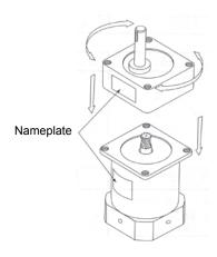
When fitting the geared motor to the application, the output shaft bearing housing can be used as a locating spiggot for mounting the unit. For square gearboxes, the fixing bolts can be used to fix the geared motor directly to the application. In this case, it is important that the motor and gearbox do not separate, which could cause damage to the motor pinion.
