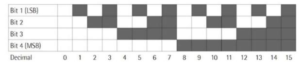
Figure 2. Binary code 4-bit representation (high logic level is represented in black)
