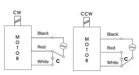
The direction of motor rotation is as viewed from the front shaft end of the motor
