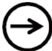
Figure 4.3 Emergency Stop Safety Disconnect symbol
