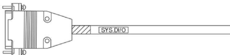
**Figure 9.2 System DI/O Extension Cord (3081425800)**
