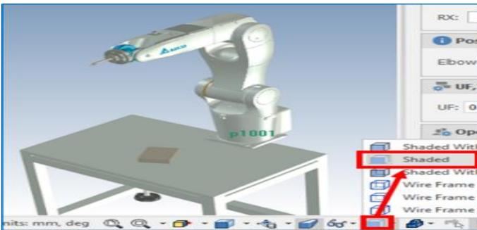
2. The robot position obtained by dragging the TriBall drag Mode cannot be used for teach and save
