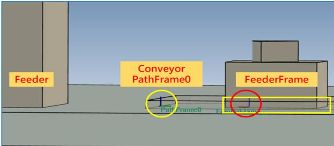
Conveyor supports in moving the work piece on the defined conveyor path frame. In simulation where user needs to move the work piece on a conveyor, built-in library function of conveyor used to configure.
