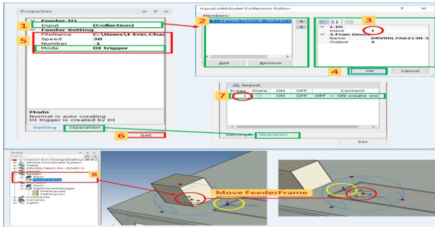
Feeder properties can define parameters of Feeder IO control, feeding speed and quantity of work pieces etc.
