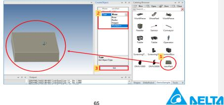
4. Work piece generation by Feeder –Work Piece anchor point to be maintained at global coordinate origin. Work piece will generate at feeder frame position added with offset distance from the global origin.
