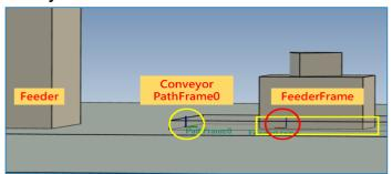
Conveyor supports in moving the work piece on the defined conveyor path frame. In simulation where user needs to move the work piece on a conveyor, built -in library function of conveyor used to configure.
