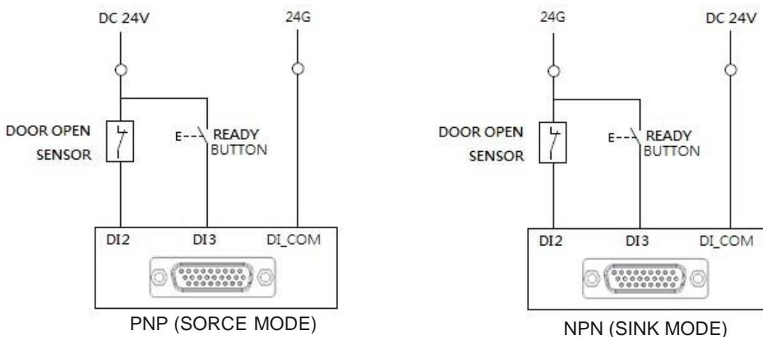
Figure 3-20 Wiring Example of the Safety Door
