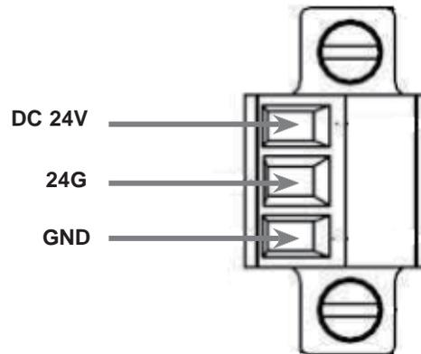
Figure 3-6 Definition for the control power terminal
