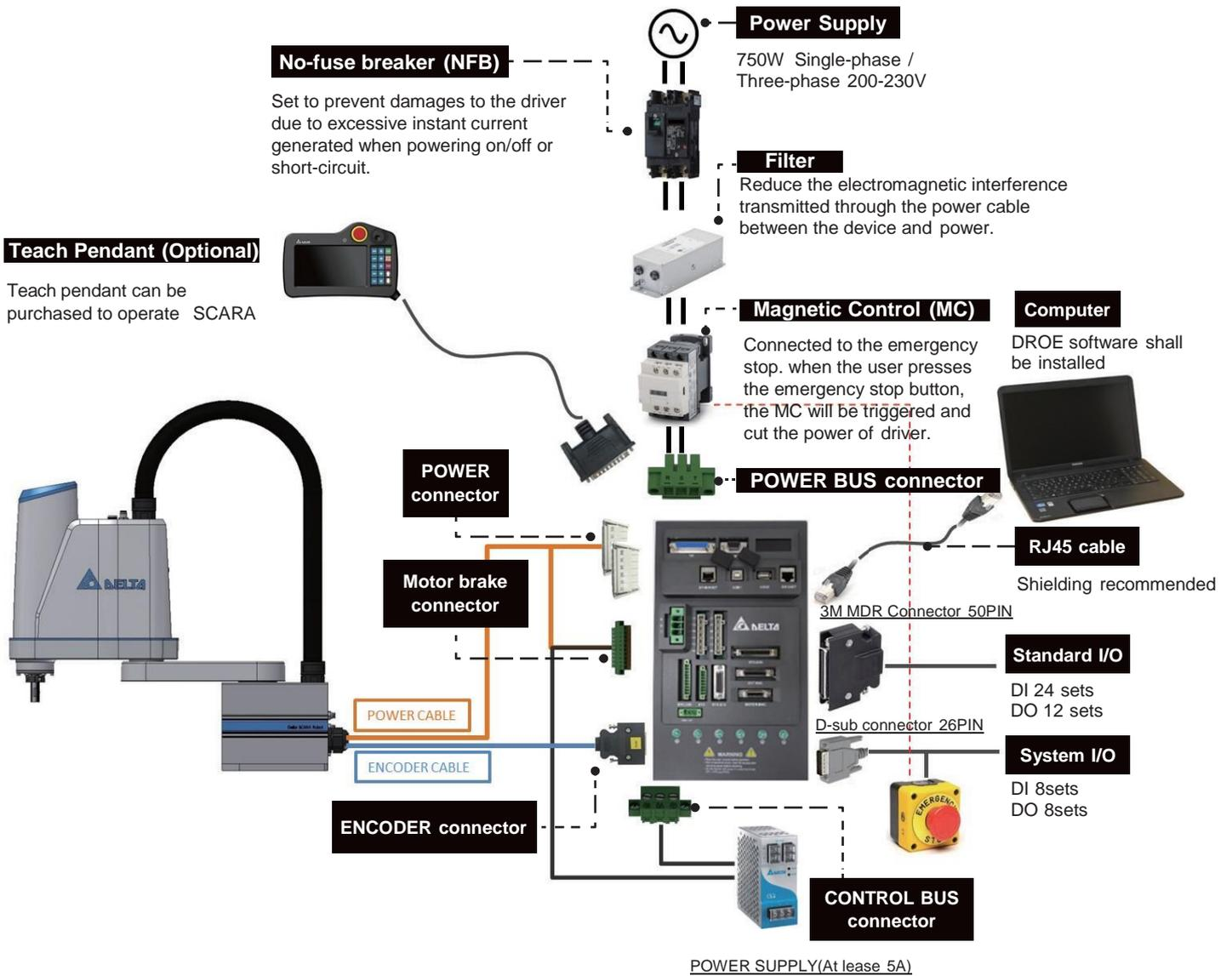
Figure 2-1 Peripheral Device Wiring Diagram
