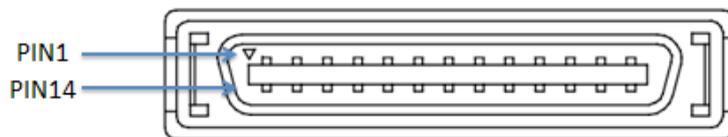
Figure 3-15 Definitions of pins on motor Encoder
