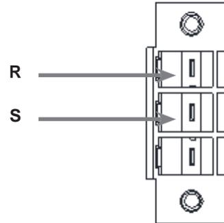
Figure 3-4 Definition for the motor power terminal
