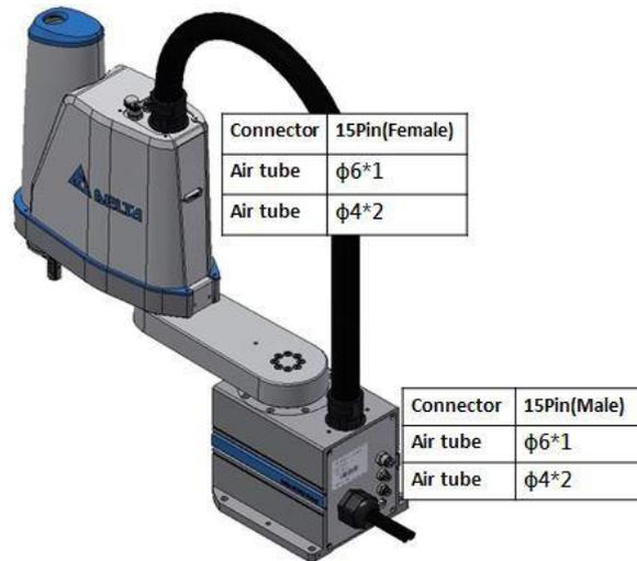
Figure 3-34 SCARA Body Connector Configuration
