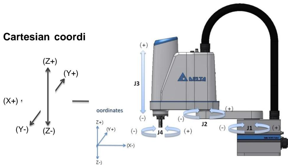
Figure 1-1 Directions of SCARA Motions
