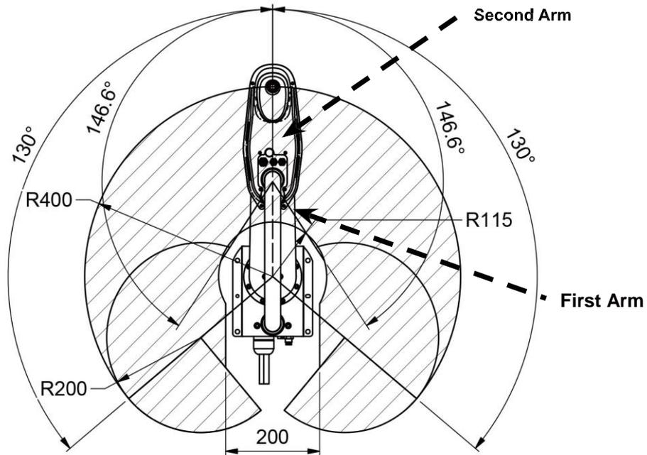
X-axis mechanical stopper position :  $133^\circ$
