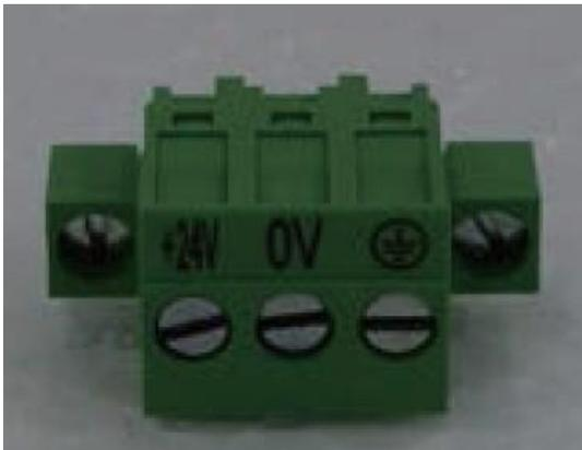
Figure 3-5 Connector for power on control circuit
