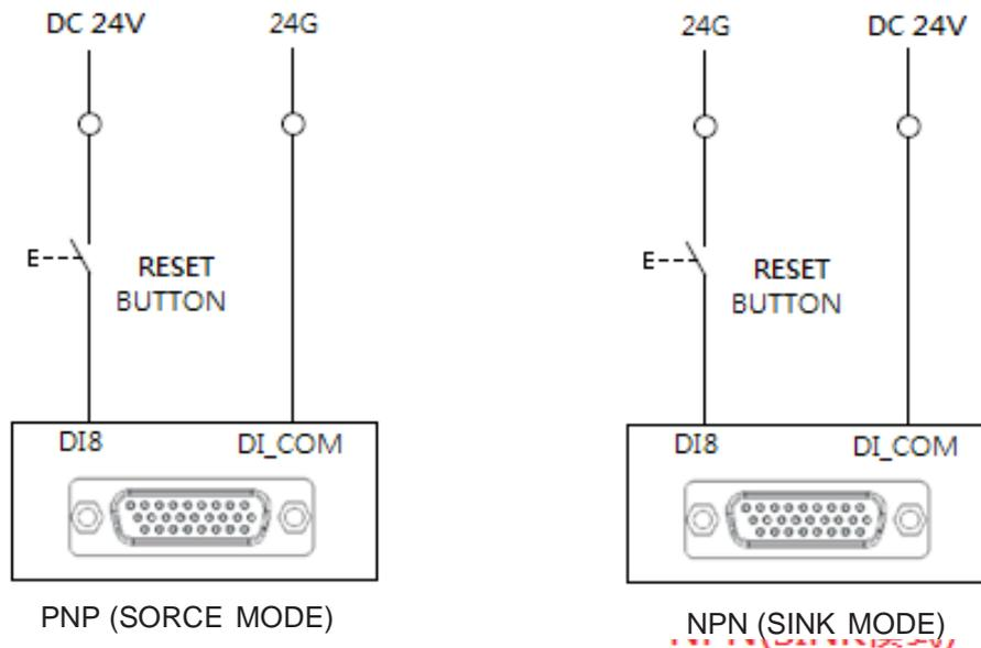
Figure 3-23 Reset Wiring Example
