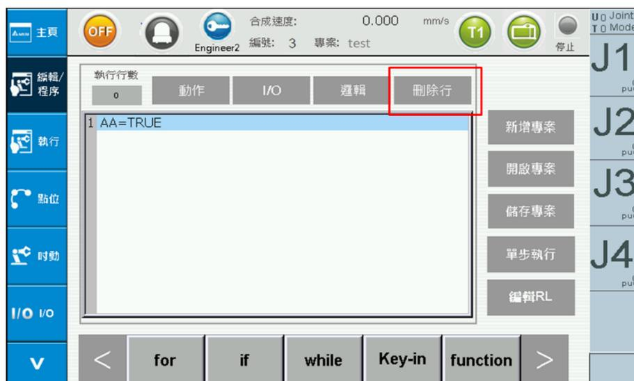
Figure 2-15 Robot Process Edit/RL - Delete Row
