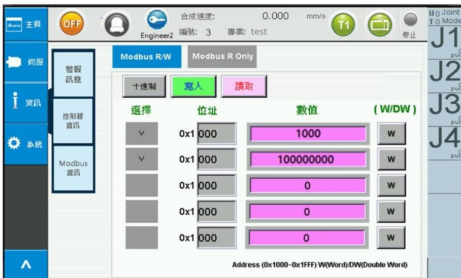
Figure 2-43 Modbus Information – Users Can Read Modbus Address Information Manually
