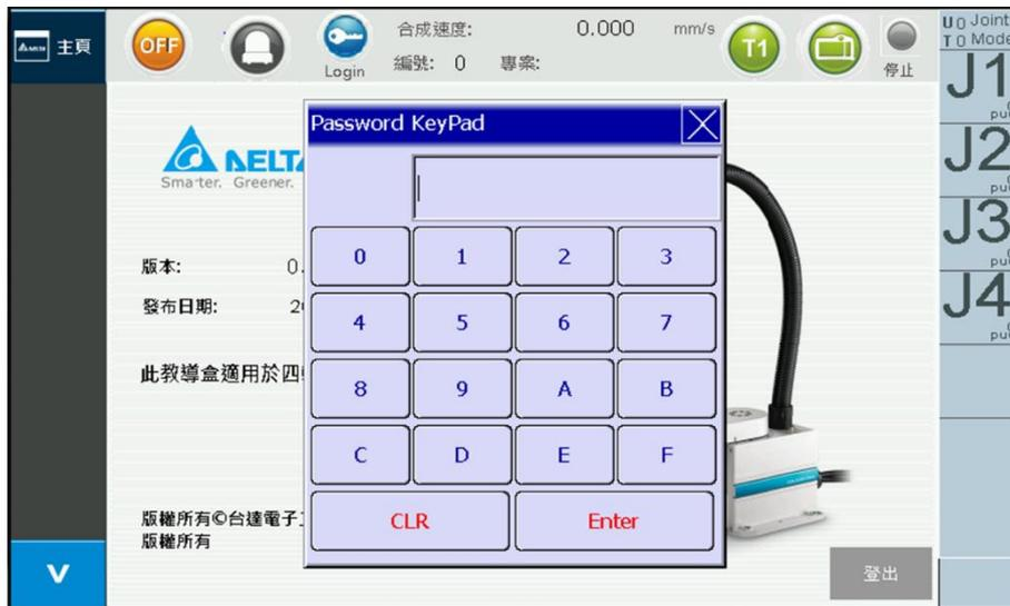
Figure 2-3 Main Screen - Logged In (robot operation mode T1, TP operation mode Enable)
