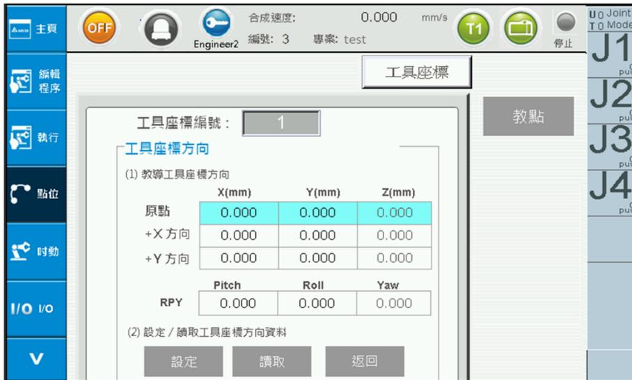
Figure 2-31 Point Information - Tool Orientation Calibration
