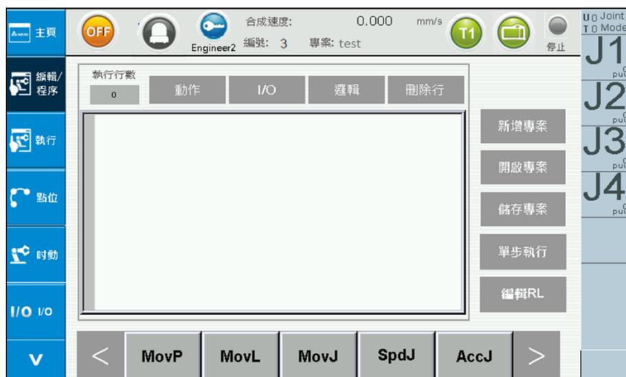
Figure 2-11 Robot Process Edit/RL - Select Input Position
