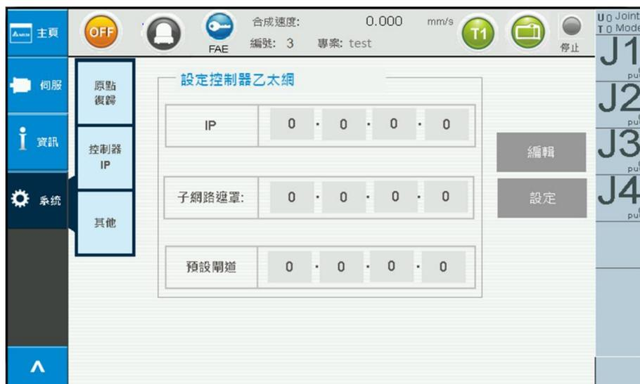
Figure 2-46 System Setting - Controller IP
