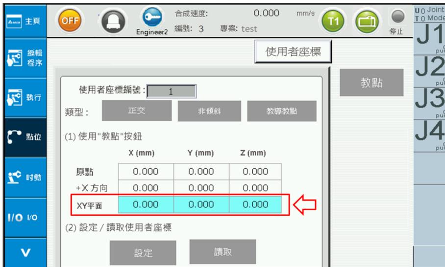
Figure 2-23 Point Information - User Coordinate XY Plane Point Setting (determine +Y direction)
