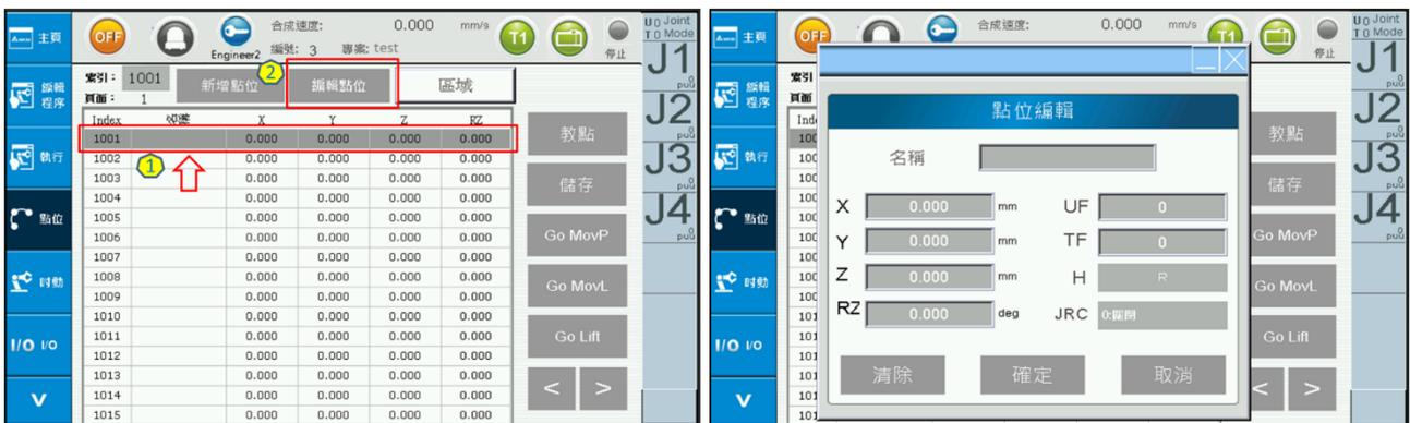
Figure 2-20 Point Information - Users Set the Local Point Parameters Manually
