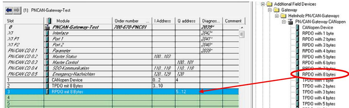
The sequence of the TPDO and RPDO entries in the configuration can be selected as desired. All TPDO and RPDO entries following a CANopen® device entry belong precisely to this device.
