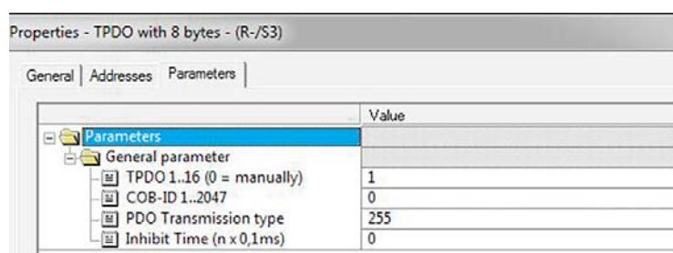
**PDO 1..16:** With the specification of the PDO number (1..16), all necessary settings for the PDO are made automatically by the PN/CAN at the start. The default COB-ID of the slave is set, the transmission type and the inhibit time are set, and the PDO activated.
