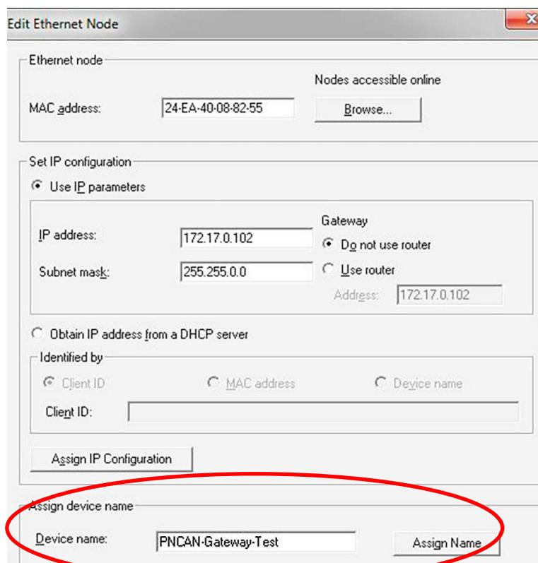
If the PN/CAN gateway has been assigned the correct PROFINET name, it is recognized by the PLC and configured.
