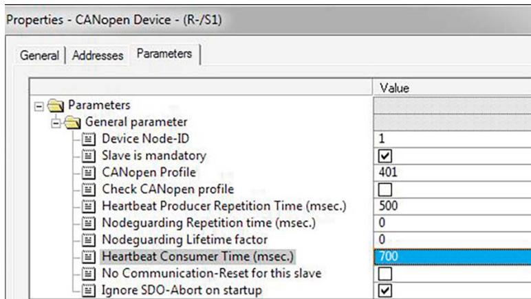
The **device node ID** of the CANopen® slave must be set absolutely correctly and uniquely.
