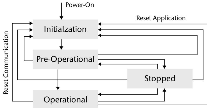
With the NMT command "Operational" [COB-ID: 000<sub>hex</sub> / data (2 bytes): 01<sub>hex</sub> node ID], a CANopen® device can be switched to the operational status. Once in the Operational state, the coupler's process data will be enabled (RPDO/TPDO communications will be running). The options available for making changes to SDOs may be limited.
