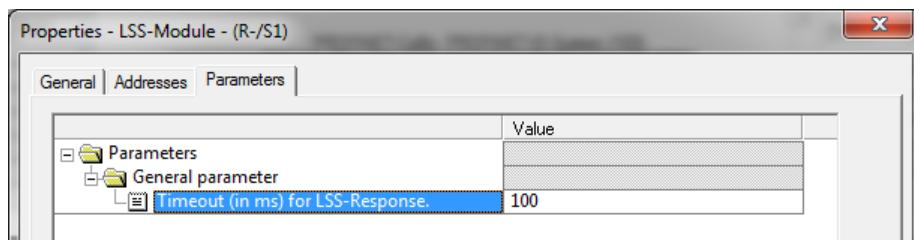
In order to carry out the LSS functions on the CAN bus, these must be programmed in the PLC. To this purpose, the LSS module makes available the following command interface in the IO map.
