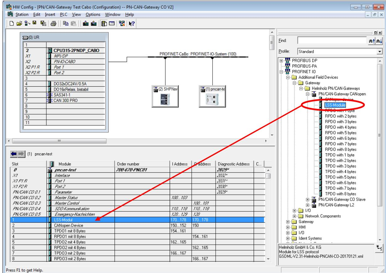
The LSS module has as its only parameter the timeout time for responding to LSS requests:
