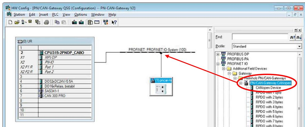
By calling up the object properties, the PN/CAN gateway should be assigned a unique PROFINET name and the IP address be checked for plausibility.
