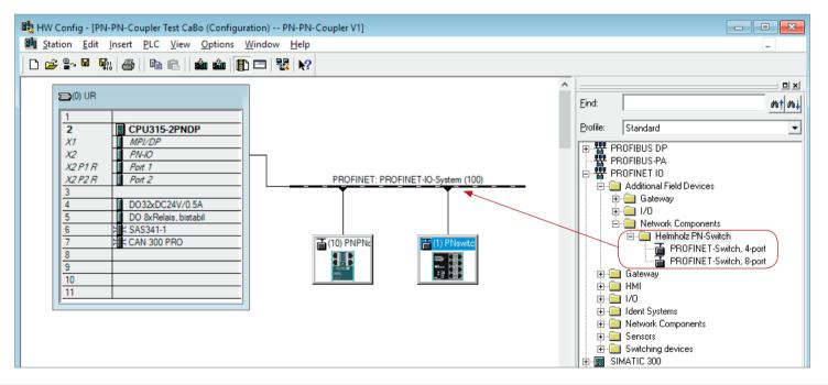
By calling up the object properties, you can assign the PROFINET switch a unique PROFINET name and check the IP address for plausibility in the project.
