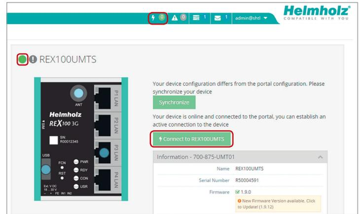
The connection status with the REX 100 is represented with an orange LED ●. In order to end the connection of a remote access, please click the in the meantime yellow and animated connection button and then confirm the disconnection of the remote connection.
